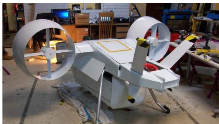
Sky Hopper in the workshop being prepared for display. The underslung cargo module sub-system is clearly visible.
